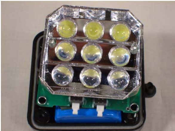
The reflector with the LEDs
